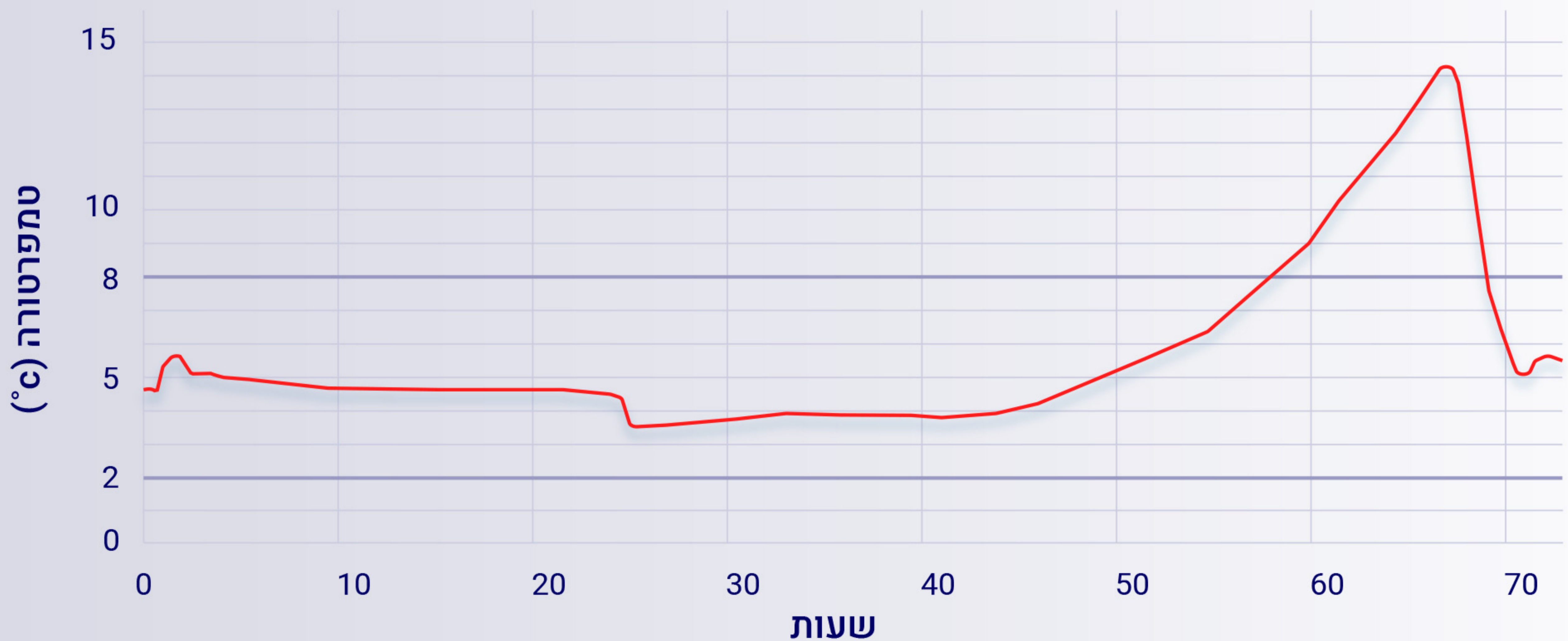
Refrigerator Power Off test Chamber Thermal Mapping
